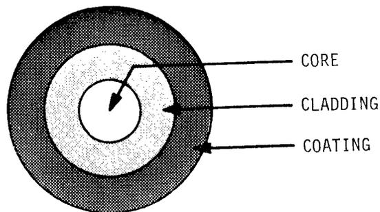
(1) Core. The core is the central part of the fiber through which light is transmitted. The amount of light coupled into a fiber is directly proportional to the square of the diameter of its core.
