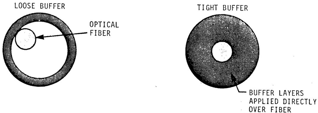
(1) Loose Buffer. In loose buffer construction, the fiber is contained in a plastic tube that has an inner diameter considerably larger than the fiber itself. The loose tube isolates the fiber from the exterior mechanical forces acting on the cable. By controlling the amount of fiber inside the tube, the amount of allowable temperature variation can be increased and, therefore, the degree of attenuation over a temperature range is minimized.
