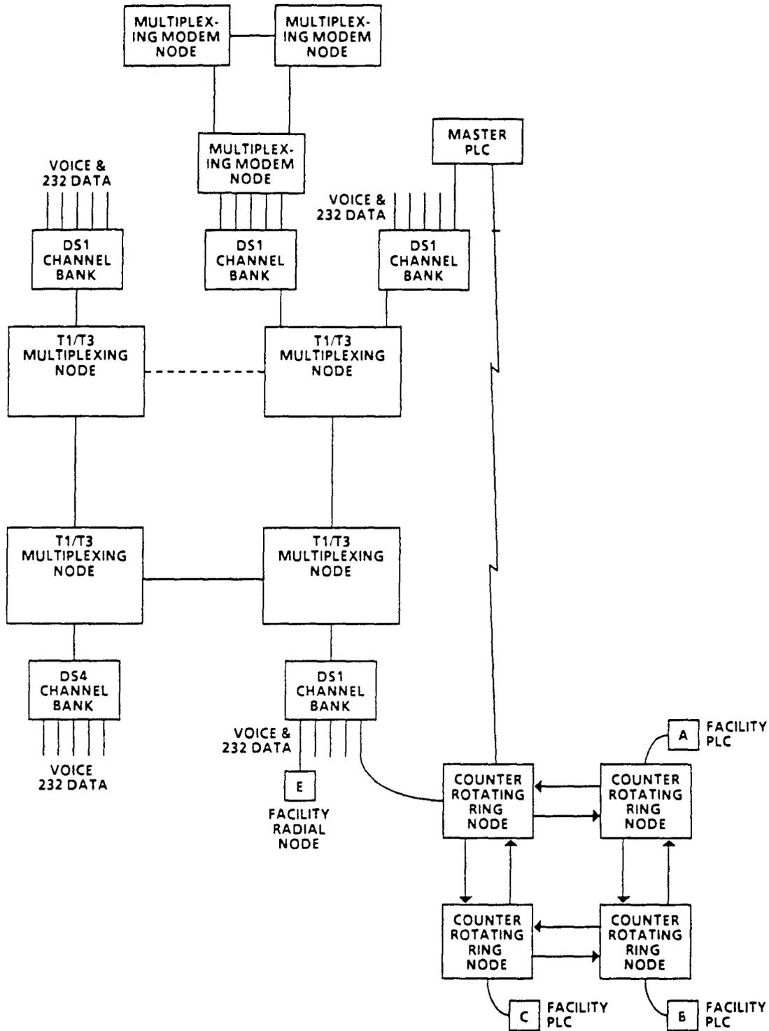
FIGURE 1-2. T-CARRIER NETWORK w/Counter-Rotating Rings and Point-to-Point Elements
