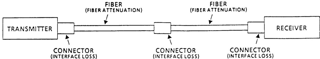
(1) Optical Fiber Loss. Light is subject to transmission losses associated with a propagation medium.
