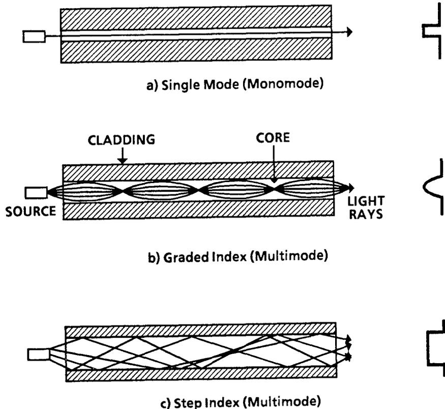
a. Step-Index. Step-index multimode fiber derives its name from the distinct, step-like difference in the refractive index of the core and the cladding. Common step-index fibers have core diameters of 100, 200 and 300 microns. Step-index fiber limits the system bandwidth to approximately 20 MHz\*km
